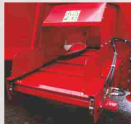
Model VLX-K has a chain conveyor with side-shift at front.
